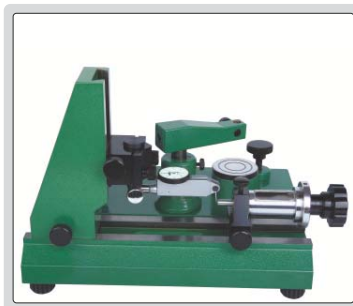
Inspect accuracy of test indicators
